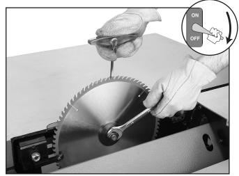
Figure 49. Replacing the main blade.
